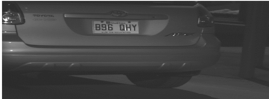
In the ALPR image above, the B could be read as an 8 and the Q as an O.
