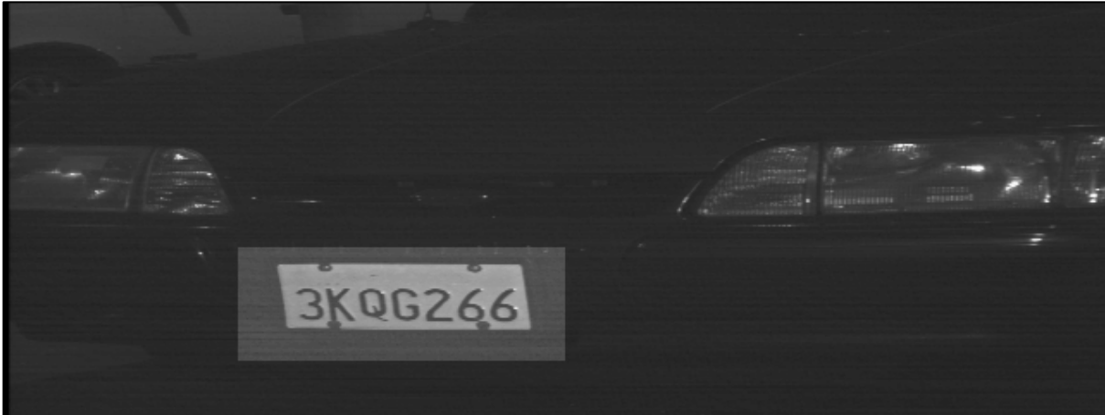
An example of a license plate that has been located in the larger vehicle image captured by an ALPR camera.
