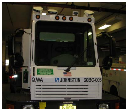
ALPR cameras mounted on top of a street sweeper aid in street maintenance.
