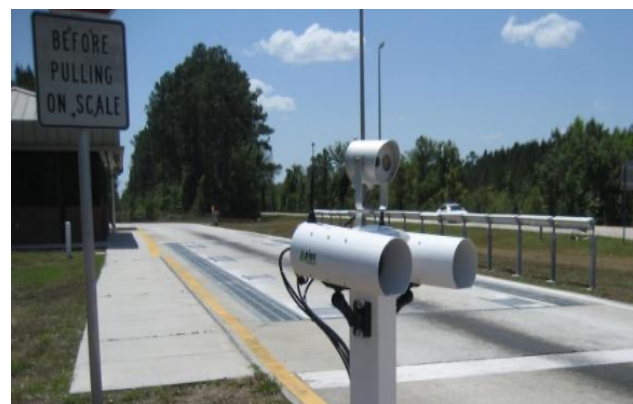
Automated license plate recognition camera in use at a roadside truck scale.
